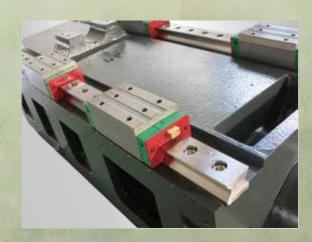
All axes adopt roller type linear guide ways that support heavy cutting, fast movement and lower wear.
