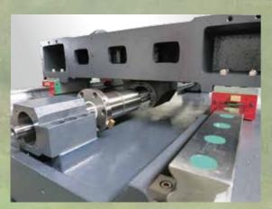
X / Y / Z axes direct driven by AC servo motor to ensure that the high-speed axial load, which still provides the best dynamic accuracy and fast acceleration and deceleration capacity.
