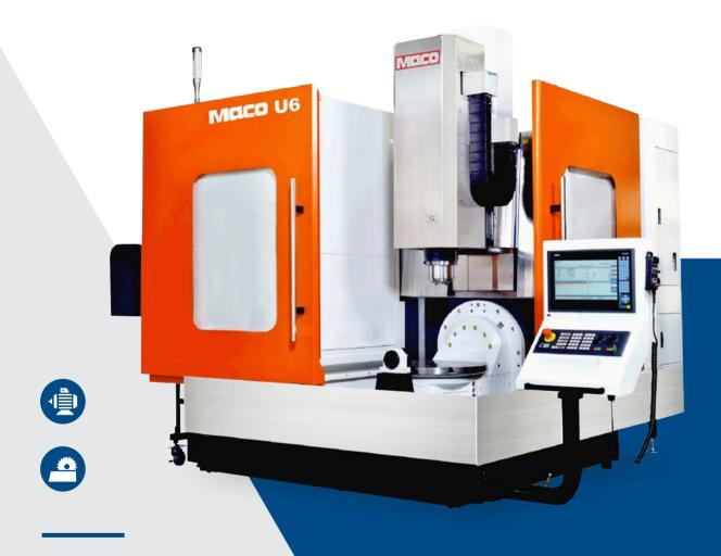
All mechanical parts are guided by Finite Element Analysis. The onepiece high tension casting structure allow column and saddle to be perfectly matched. The X and Y axes are combined with cross-slide design to ensure high stability and machining accuracy.
